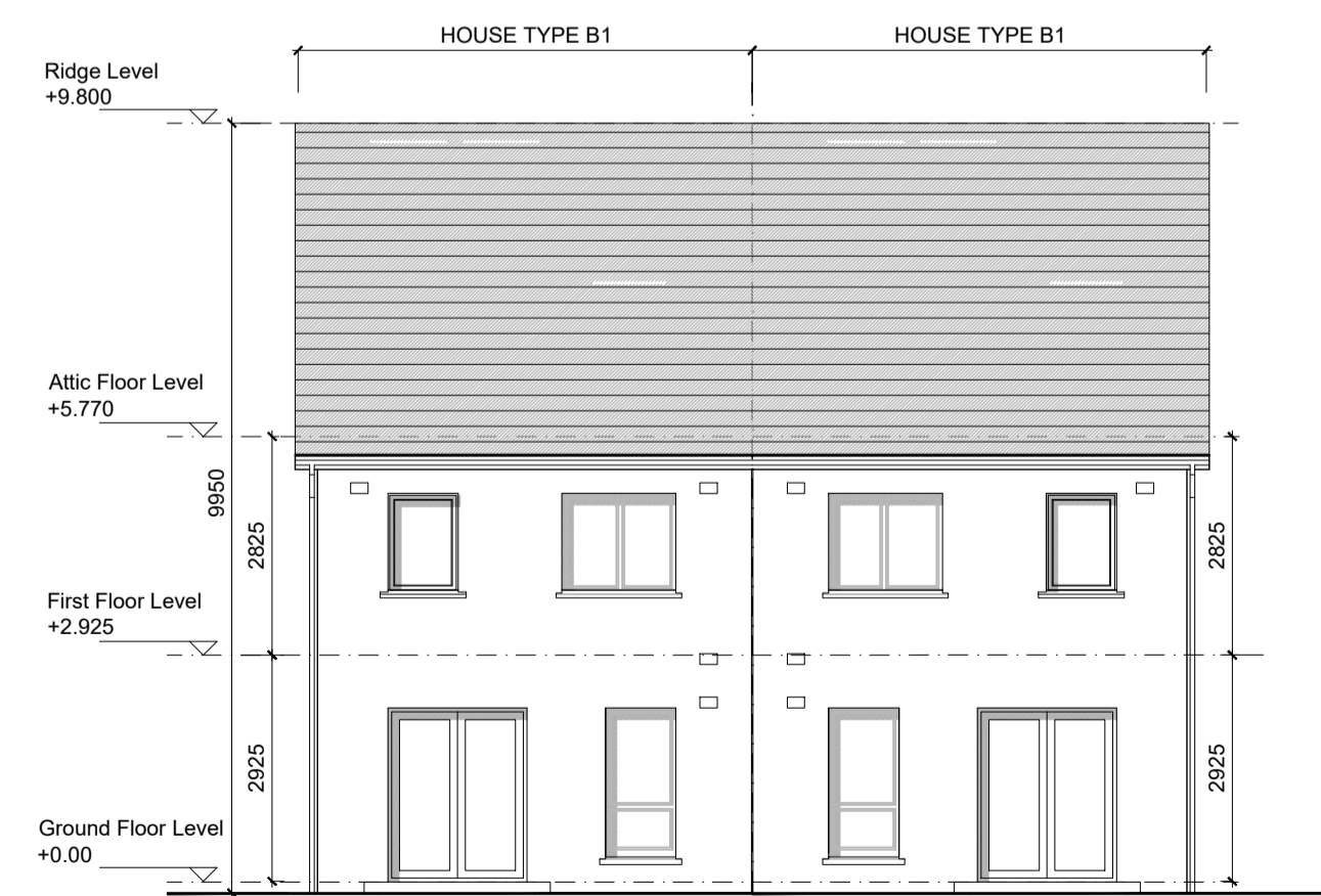
REAR ELEVATION (Type B1-B1) Scale 1:100
