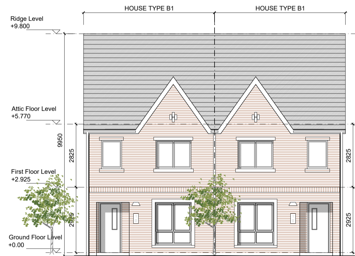
FRONT ELEVATION (Type B1-B1) Scale 1:100
